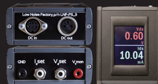
LNF-PS_3 (Constant current power supply with display for 1 LNA)
